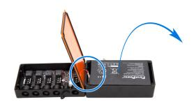
3. Insert the new batteries in the control box and connect the plus and minus cables. Please note! Sparks may occur when plugged in; wear goggles.
