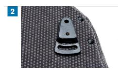
3. To prepare for the threaded inserts (D), drill a 6 mm hole. To be sure the hole is in the right place, drill through the upper hole in the mount (G).
